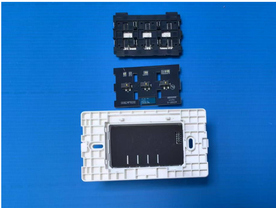
Open view of AS7A-22W (as representative for smart full touch controls switch)
